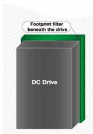
Drive mounted on an external footprint filter
